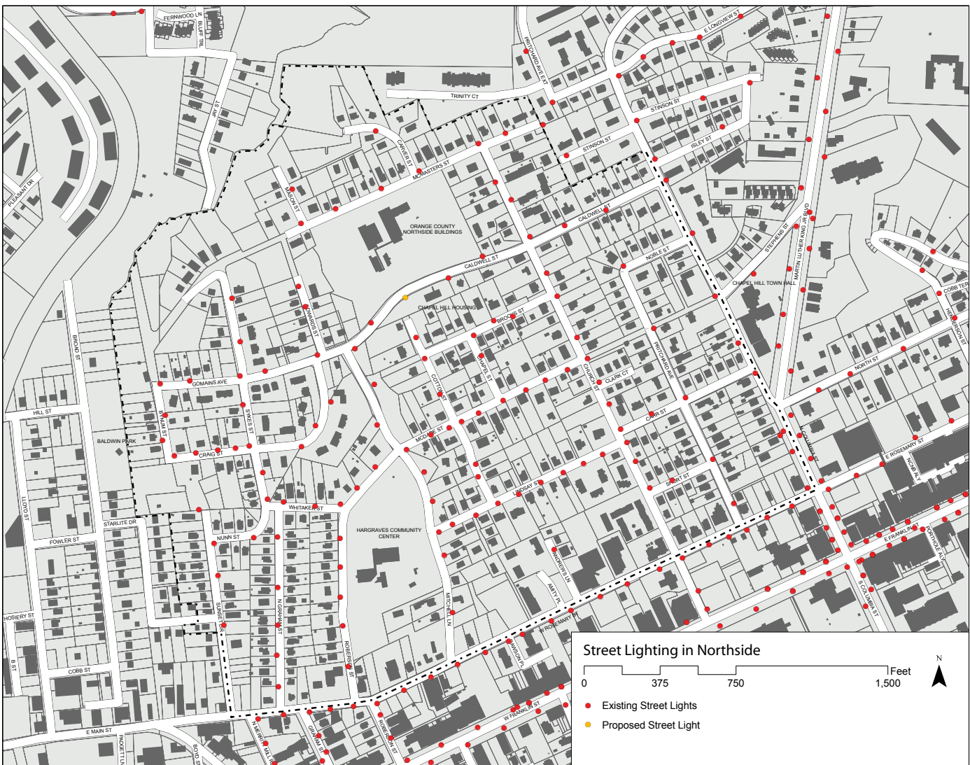
Figure G: Streetlight Location in Northside
