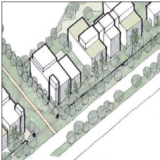
Diagrammatic Massing of Campus Frontage with Landscape Building setbacks provide sun and views into midblock areas
