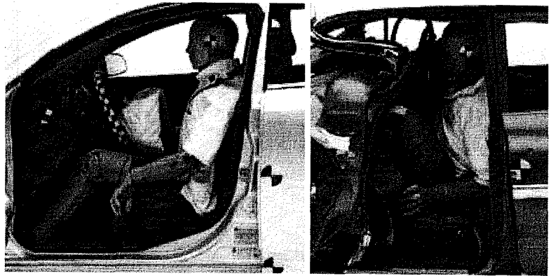
In the crash test involving the two Chevrolets, the 2009 Malibu's occupant compartment remained intact (above left) while the one in the 1959 Bel Air (right) collapsed.
