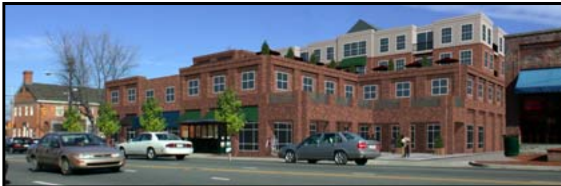
Computer illustration showing suggested building height of 2 stories at street stepped up to 4 stories in interior.
