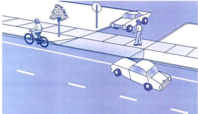
**Maintaining sidewalks at grade across driveways helps slow turning vehicles and reinforce pedestrian right-of-way. (photo, Oregon Bicycle and Pedestrian Plan)**
