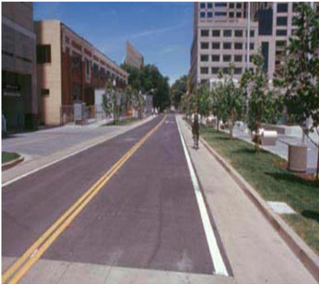
**Different paving treatments such as this concrete bike lane may enhance conspicuity of bicyclists and visually narrow the roadway. (Photo, D. Burden)**
