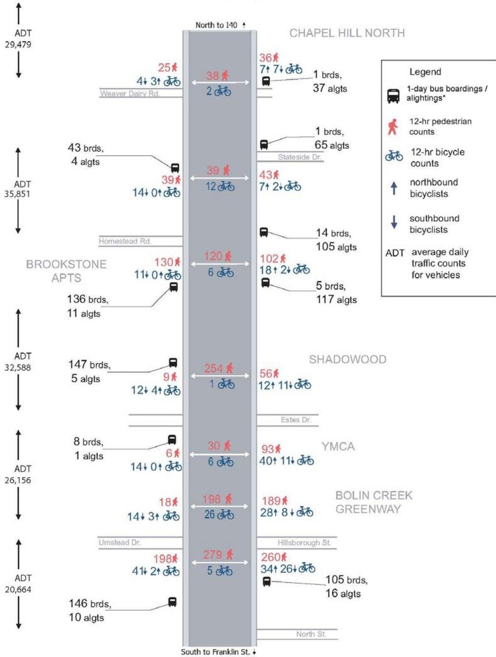
**Figure 7. Schematic diagram of corridor (not to scale) with recent counts of motor vehicle volumes (ADT), transit use, and pedestrian and bicycle activity. (Select data are shown. All counts from fall, 2003.)**
