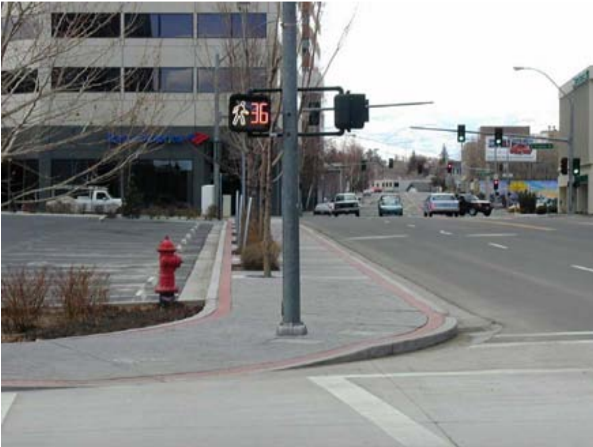
Figure 10. Pedestrian countdown signals can help pedestrians understand when they should begin crossing.
