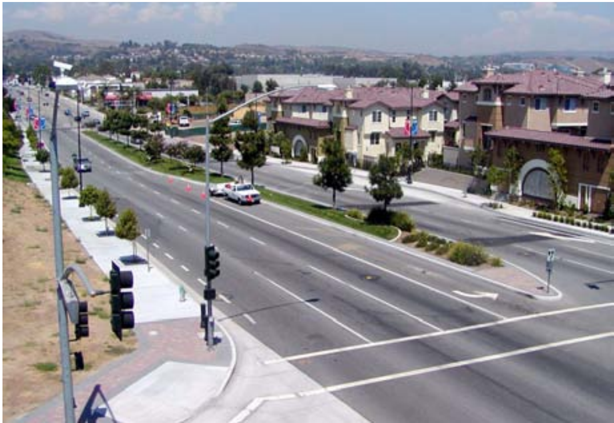
Figure 7. Well-designed pedestrian crossing islands contribute to safer pedestrian crossings at intersections.
