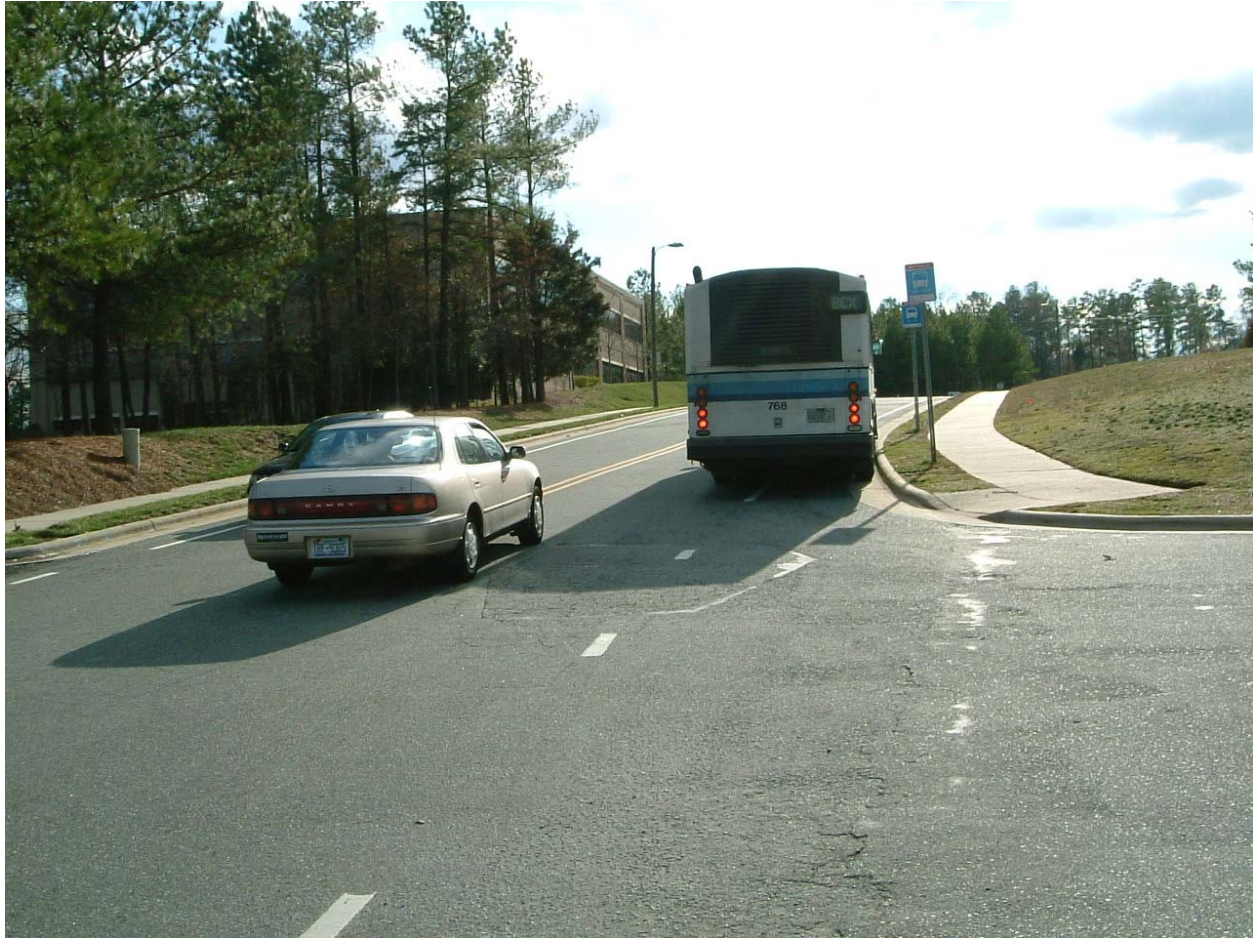
Photo 2: The parked bus prevents vehicles passing if there is oncoming traffic, as in this photo. As the bus fills all of the bicycle lane and the road, any car passing the parked bus from behind must cross the double yellow lines. Visibility up the hill is poor.
