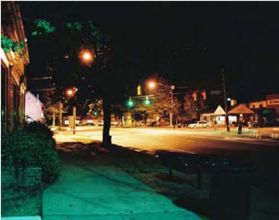
Existing fixtures in Chapel Hill use outdated mercury vapor lamps, which have lower light output per wattage than other types of light fixtures, such as the more common metal halide lamps. Metal halide lamps cast a brighter, whiter light than the blue-hued light emitted from mercury vapor lamps.
