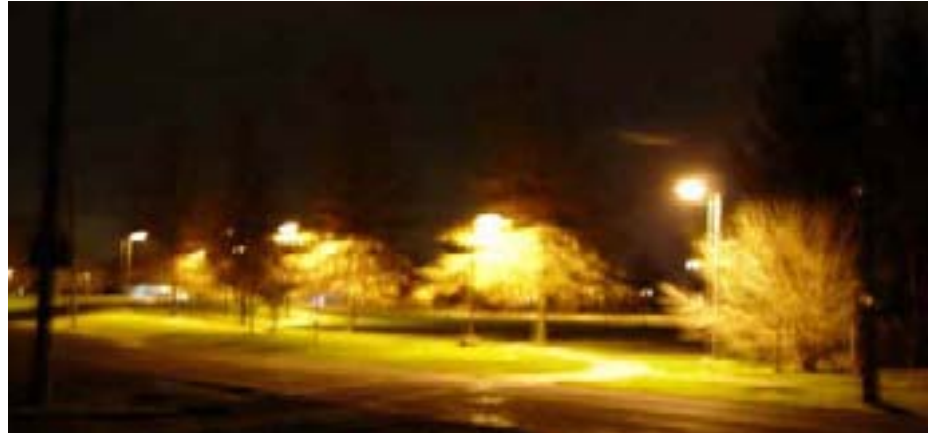
Full cutoff lights direct all light downward, maintaining a brightly illuminated path without casting unnecessary light elsewhere. Note that light does not extend into upper portion of the trees above each fixture. ( www.nightwise.org )
