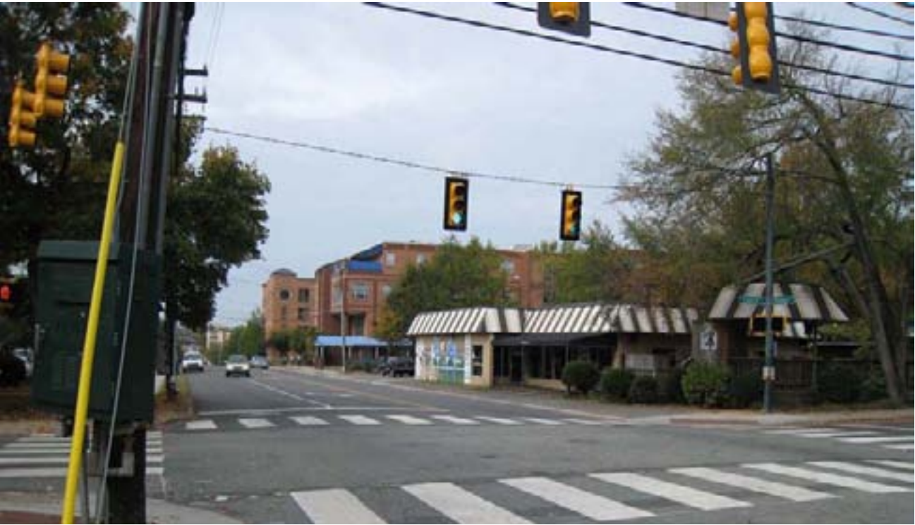
The majority of traffic signals in Downtown Chapel Hill are cable-supported. Above is an example of cable-supported traffic lights at the intersection of Rosemary and Church Streets.
