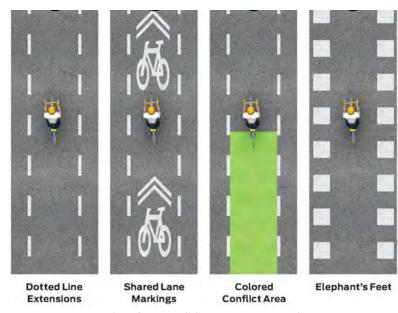
Examples of various bike intersection markings Source: NACTO Intersection Crossing Markings Design Guidance
