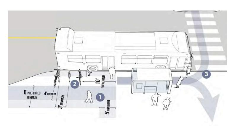
Guidance for placement of bicycle parking at a typical transit stop. (Source: NACTO Transit Street Design Guide)
