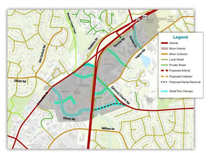
**Figure 11.** Existing streets and proposed changes to the street network in the Ephesus-Fordham District. New internal streets in the district (shown in grey) will occur with redevelopment according to the Block Perimeter and Regulating Plan
